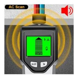
• The Wire Warning feature indicates the presence of live, unshielded electrical wiring up to 2 inches (51 mm) deep. This wall scanner always detects and indicates Live AC Wire in all modes. The Wire Warning Detection Icon flashes when live, unshielded wires are detected.
